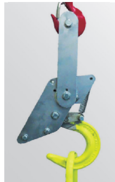
1. The hook engages with the load.
