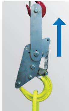
2. The load is lifted, the hook locks, preventing load from falling.
